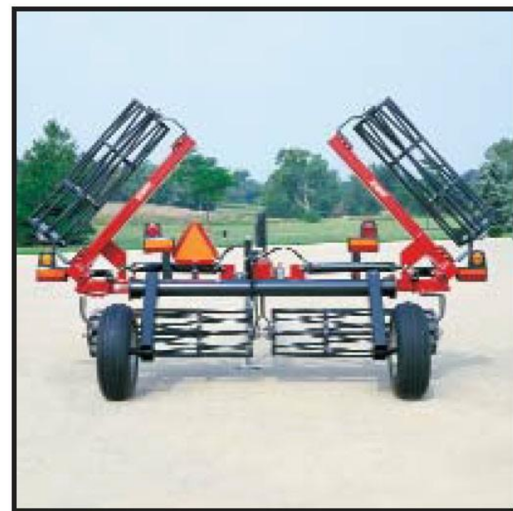
A 20' and 25' crumbler will fold to a narrow 13' transport width
